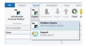
The Modbus Master is an IPEmotion system that represents a connection to the Modbus system. The Modbus system can be connected via TCP or serial connection to the PC. After selecting the **Modbus Master** you have to define the connection to the Modbus system in the tab **Connection**.
