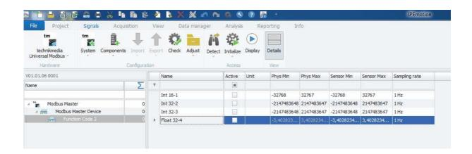
**Every function code group has an address range without gaps**. That means that the first value has the start address of the function code group. If the value is a bit value, a 16 bit integer or a 16 bit unsigned integer, the address of the next value in this function code group has the next address. If the value needs 32 bit, the address of the next value is the next but one. The following table shows the addresses of the example value list above.
