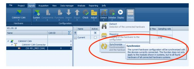
Synchronization will not remove configured current clamps from IPEmotion. The system scans all CAN busses and adds all newly found current clamps whose serial numbers are not listed in the existing configuration.
