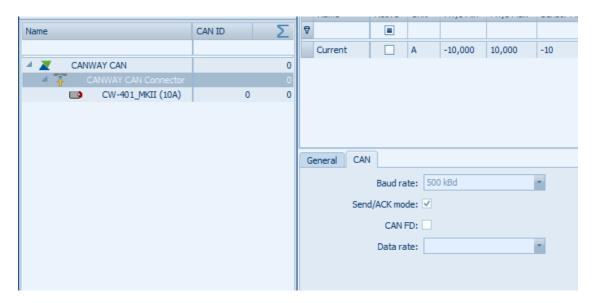
The baud rate displayed in the **CAN** tab corresponds to the CAN bus baud rate of the connected CAN adapter.
