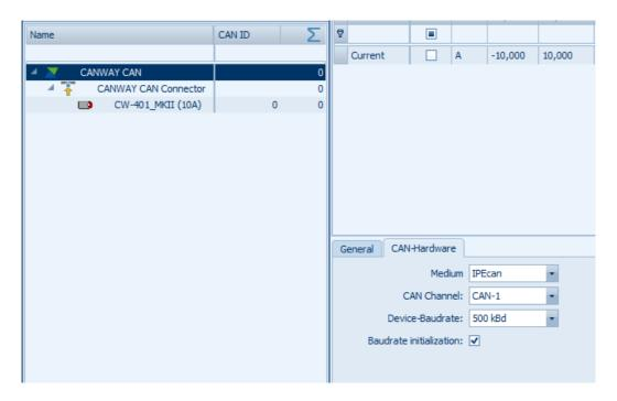
The following parameters can be configured in the **CAN-Hardware** tab:
