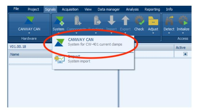
3. By clicking on **CANWAY CAN**, IPEmotion adds a **CANWAY CAN** system to the tree structure. At the same time the **CANWAY CAN** system is extended by a **CANWAY CAN Connector** as a subelement. Click on the **CANWAY CAN Connector** and unlock the **Components** button.
